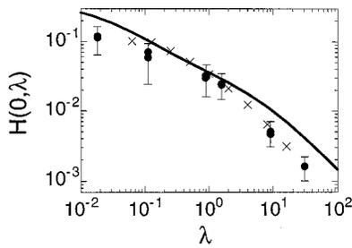
FIG. 9. Plot of the rescaled experimental (Ref. 11) (solid circles) and numerical (Ref. 14) ( $\times$ 's) minimum radius  $H(0, \lambda)$  as a function of the viscosity ratio  $\lambda$  and the result of the stability argument (solid line) presented by Cohen *et al.* (Ref. 11).
