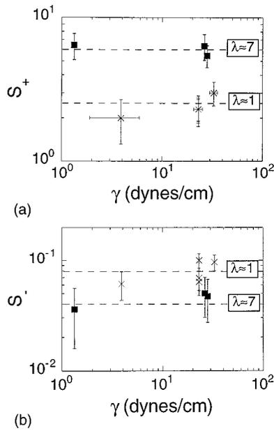
FIG. 5. Plots of the slopes (a)  $S_+$  and (b)  $S_-$  as a function of the surface tension  $\gamma$ . Each symbol corresponds to fluid systems with approximately the same viscosity ratio  $\lambda$  (within 30%) and exactly the same nozzle diameter  $D$ . For each of these, both  $S_+$  and  $S_-$  show no dependence on  $\gamma$ . The horizontal lines running through the data sets are guides to the eye.
