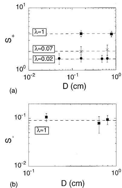
FIG. 4. Plots of the slopes (a)  $S_+$  and (b)  $S_-$  as a function of the nozzle diameter  $D$ . The different symbols correspond to fluid systems with different viscosity ratios  $\lambda$ . For each fluid system with fixed  $\lambda$  both  $S_+$  and  $S_-$  show no dependence on  $D$ . The horizontal lines running through the data sets are guides to the eye.
