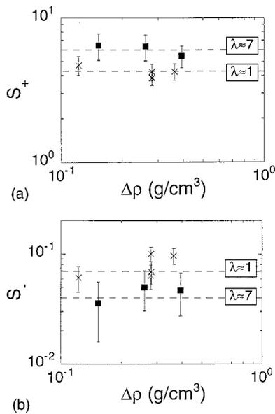
FIG. 6. Plots of the slopes (a)  $S_+$  and (b)  $S_-$  as a function of the density mismatch  $\Delta\rho$ . The fluid systems used are the same as those in Fig. 8. Each symbol corresponds to fluid systems with approximately the same viscosity ratio  $\lambda$ , and exactly the same nozzle diameter  $D$ . For these sets of fluids, both  $S_+$  and  $S_-$  show no dependence on  $\Delta\rho$ . The horizontal lines running through the data sets are guides to the eye.
